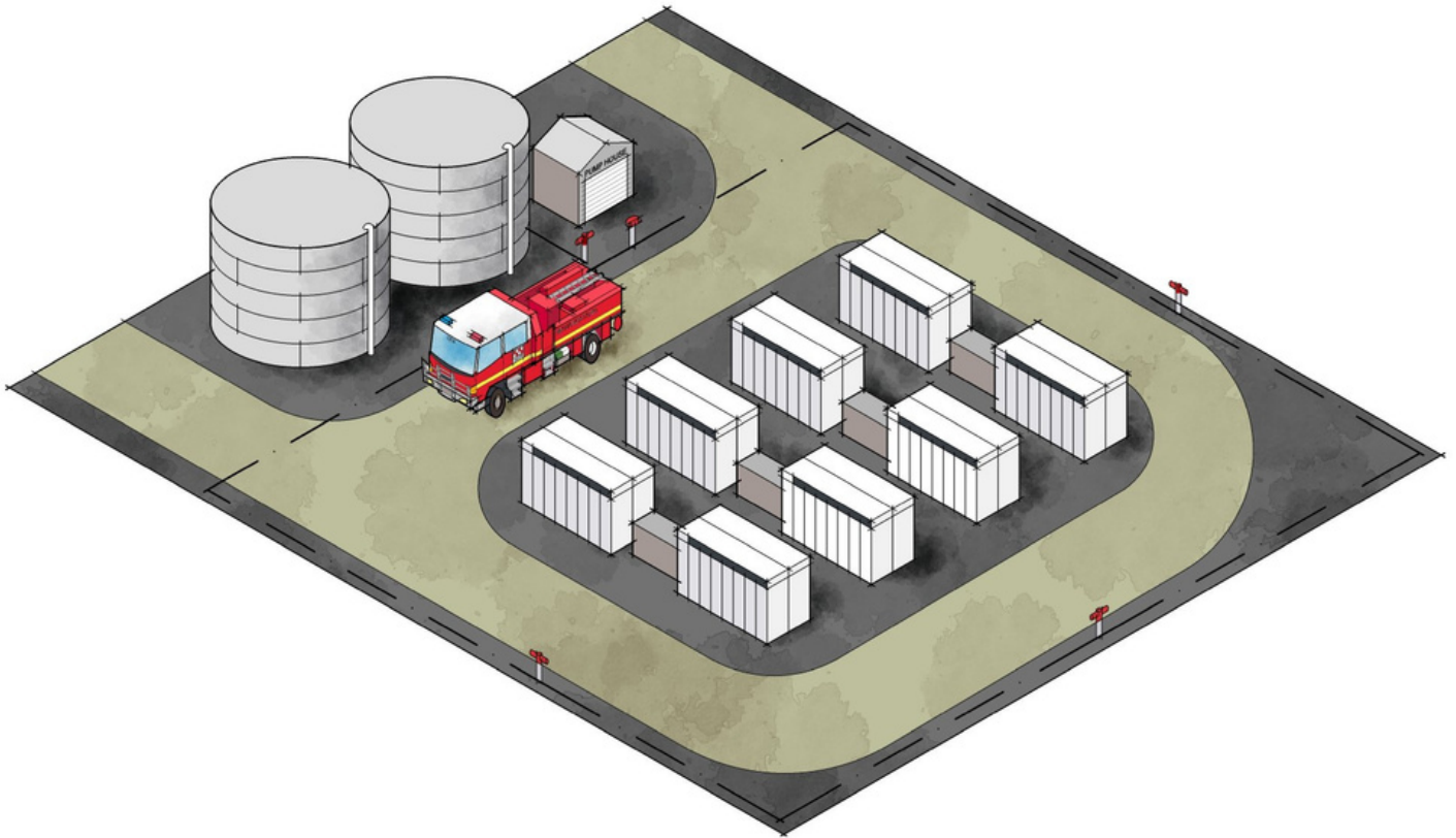
Figure 9: Best-practice arrangement of fire service infrastructure at facilities with centralised battery energy storage systems without reticulated water supply, or a reticulated water supply that does not meet the performance requirements of AS 2419.1-2021: Fire hydrant installations .
