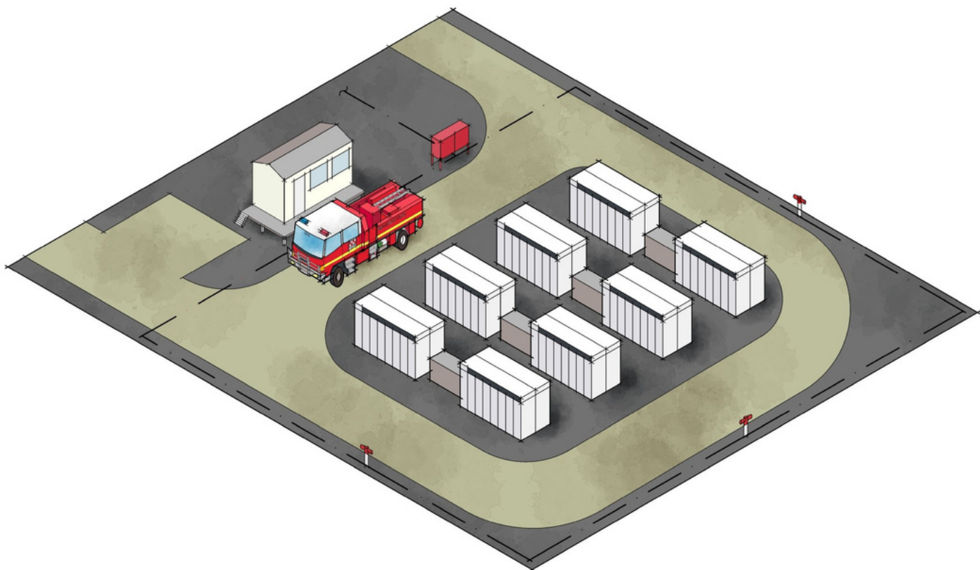
Figure 7: Best-practice arrangement of fire service infrastructure for facilities with centralised battery energy storage systems with reticulated water supply meeting the performance requirements of AS 2419.1-2021: Fire hydrant installations .
